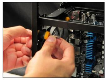
The TrueQuiet<sup>™</sup> fan has two small black clips attached to the fan's two-speed switch. With your thumb and forefinger, spread the clips while pushing from the rear of the case to remove the switch.
